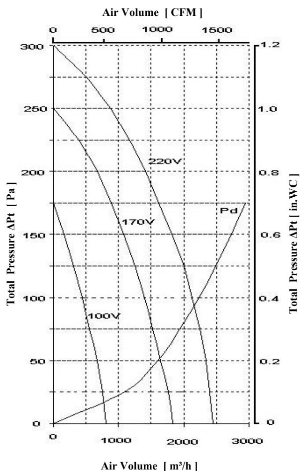
Diagram is based on standard air  $\rho=1.2 \text{ kg/m}^3$ .
